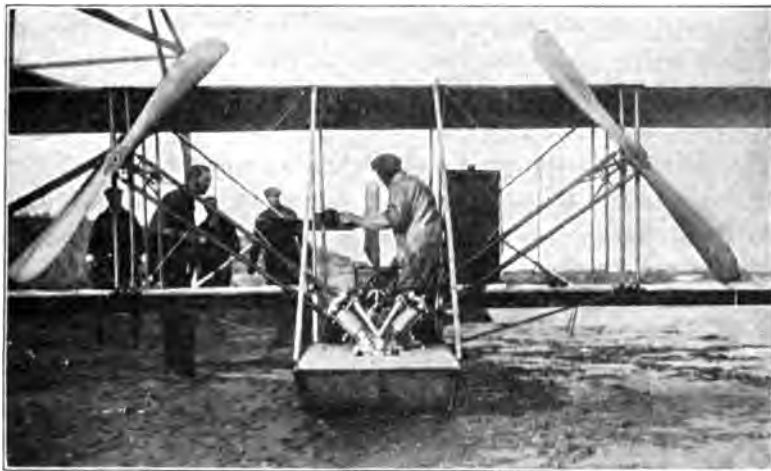
Fig. 61. Latest Model of Curtiss Hydroaeroplane Showing Two Propellers and Engine Ahead of Operator
